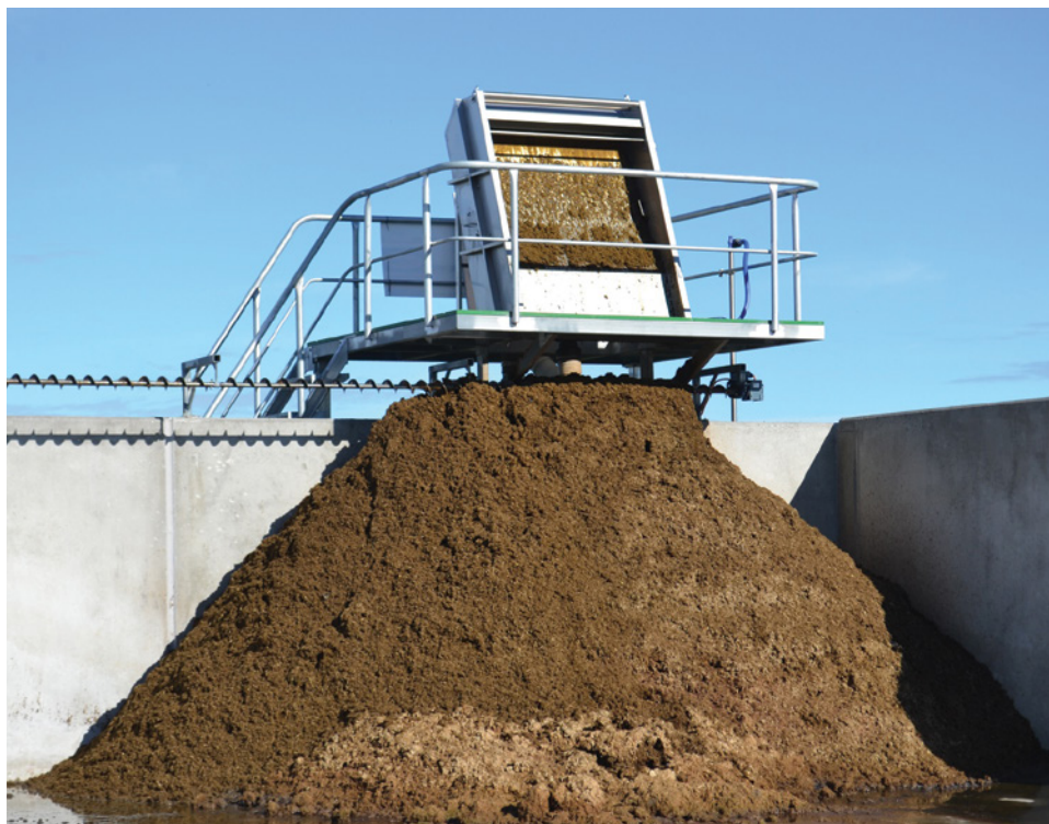
ABOVE: A major benefit to the GEA Slope Screen is the fact that it has no moving parts LEFT: This is the most reliable method in being able to meet the new cooling standards and gives farmers the peace of mind even in the heat of summer when ground water temperatures rise
